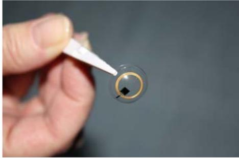
The soft contact lens like sensor, with its MEMS antenna (golden rings), its MEMS sensor (silver ring close to the outer edge), and microprocessor shown here:
